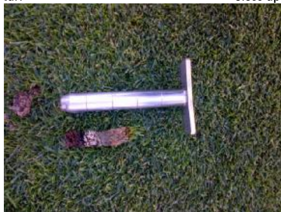
Core through upper profile with root development evident through both geotextile and shock pad
